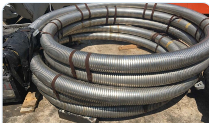
BOP Control Hose
